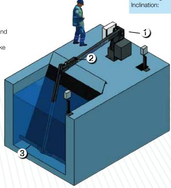
Units of the type RRH are comprised of a wide reaching articulating boom with a cleaning rake/wiper bar, attached in perpendicular direction to the flow. This boom consists of two individually jointed arms which are operated by hydraulic cylinders.
